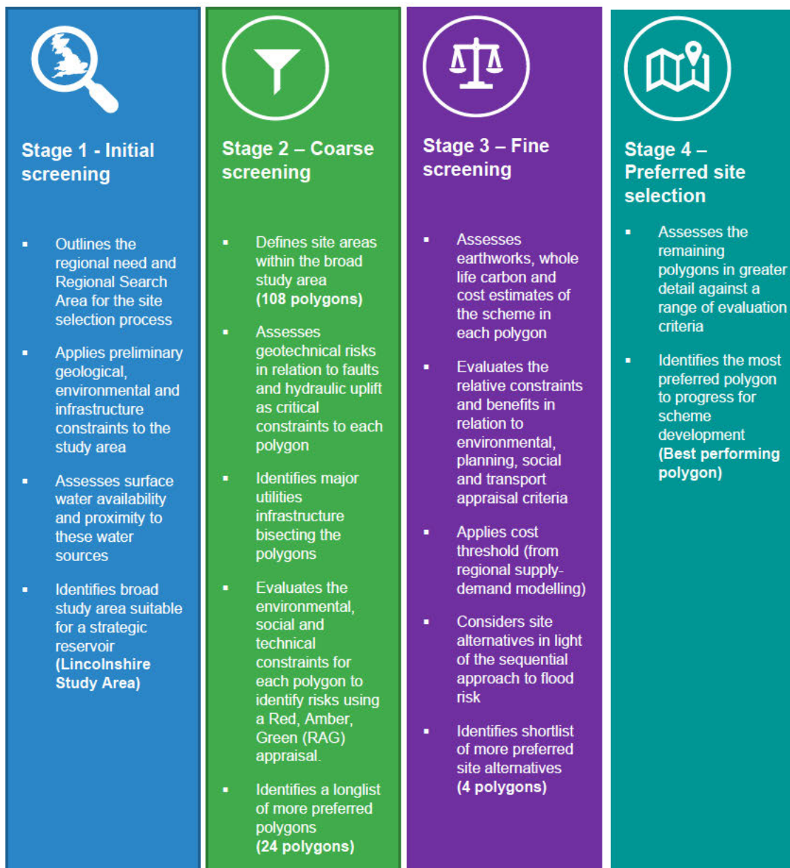
Figure 1: Staged site selection process for the South Lincolnshire Reservoir
